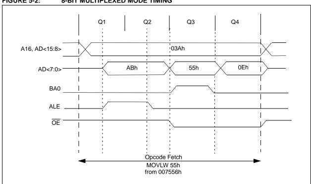
FIGURE 5-2: 8-BIT MULTIPLEXED MODE TIMING
