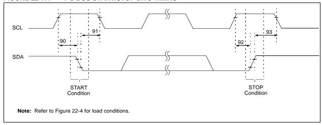
TABLE 22-16: I<sup>2</sup>C BUS START/STOP BITS REQUIREMENTS (SLAVE MODE)
