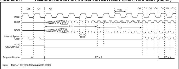
If the main oscillator is configured for HS4 (PLL) mode with SCS1 bit set to '1', an oscillator start-up time (Tost), plus an additional PLL time-out (TPLL) will occur. The PLL time-out is typically 2 ms and allows the PLL to lock to the main oscillator frequency. A timing diagram indicating the transition from the Timer1 oscillator to the main oscillator for HS4 mode is shown in Figure 2-8.
