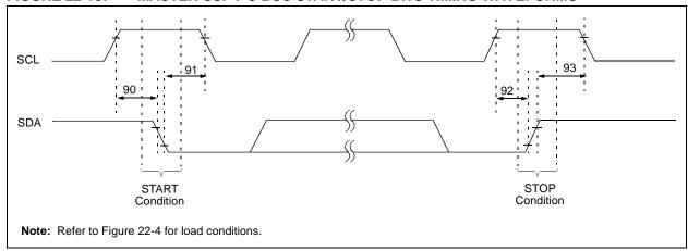
TABLE 22-18: MASTER SSP I<sup>2</sup>C BUS START/STOP BITS REQUIREMENTS
