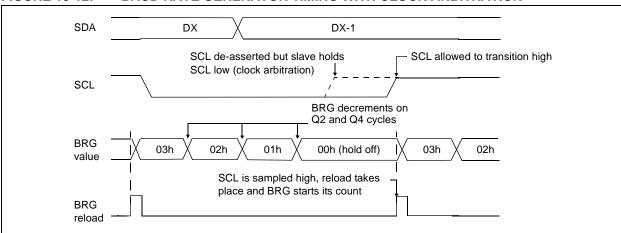
FIGURE 15-12: BAUD RATE GENERATOR TIMING WITH CLOCK ARBITRATION
