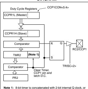
A PWM output (Figure 14-4) has a time-base (period) and a time that the output stays high (duty cycle). The frequency of the PWM is the inverse of the period (1/period).
