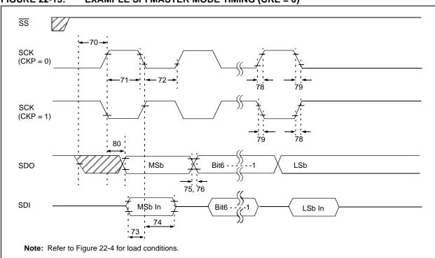
FIGURE 22-13: EXAMPLE SPI MASTER MODE TIMING (CKE = 0)
