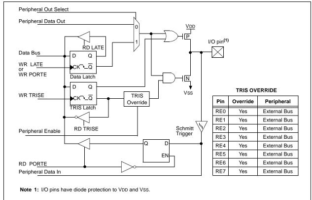
FIGURE 9-10: PORTE BLOCK DIAGRAM IN SYSTEM BUS MODE
