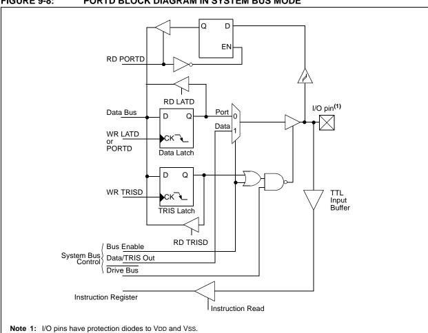
FIGURE 9-8: PORTD BLOCK DIAGRAM IN SYSTEM BUS MODE
