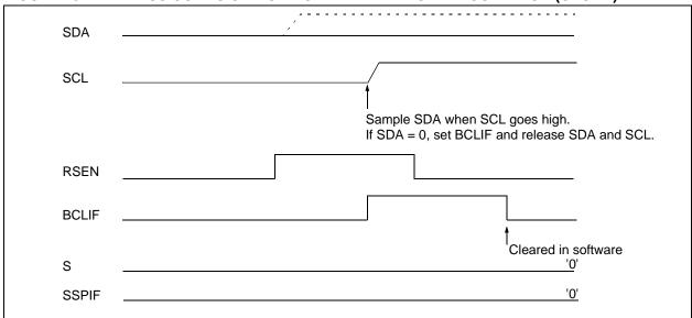
FIGURE 15-25: BUS COLLISION DURING REPEATED START CONDITION (CASE 2)
