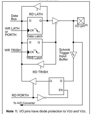
**FIGURE 9-18:** RH3:RH0 PINS BLOCK DIAGRAM IN SYSTEM BUS MODE Q D ΕN **RD PORTH RD LATD** I/O pin(1) P<u>ort</u> Data Bus D D<u>ata</u> WR LATH or PORTH
