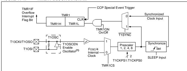
Note 1: When enable bit T1OSCEN is cleared, the inverter and feedback resistor are turned off. This reduces power drain.
