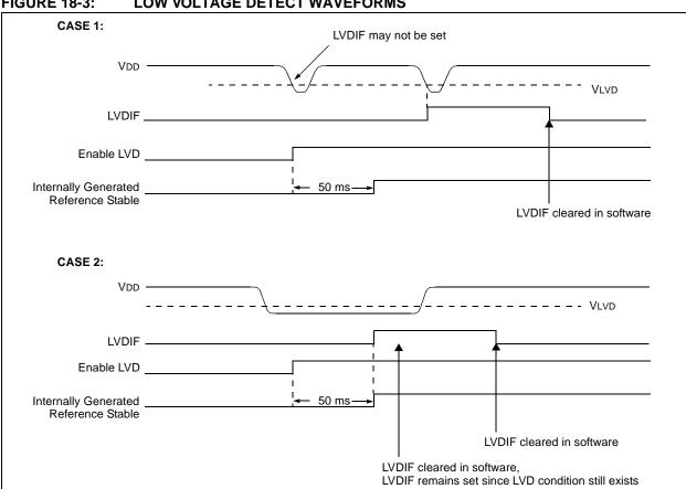
**FIGURE 18-3:** LOW VOLTAGE DETECT WAVEFORMS
