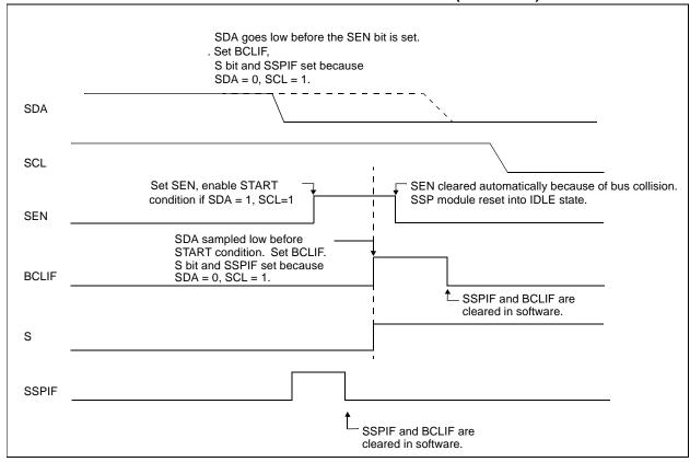
FIGURE 15-22: BUS COLLISION DURING START CONDITION (SCL = 0)
