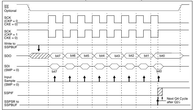
FIGURE 15-5: SPI MODE WAVEFORM (SLAVE MODE WITH CKE = 1)
