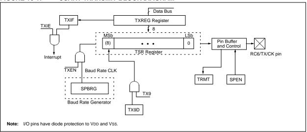
FIGURE 16-2: ASYNCHRONOUS TRANSMISSION
