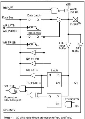
To enable weak pull-ups, set the appropriate TRIS bit(s) and clear the RBPU bit (INTCON2 register).
