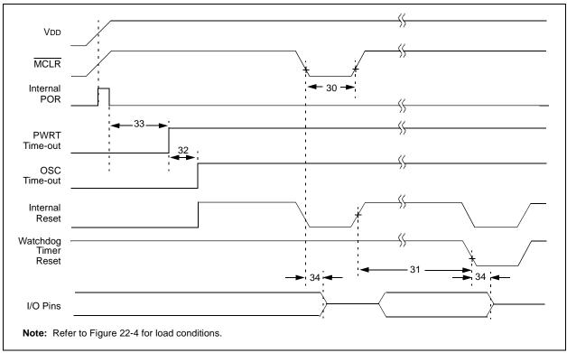
TABLE 22-9: RESET, WATCHDOG TIMER, OSCILLATOR START-UP TIMER, POWER-UP TIMER AND BROWN-OUT RESET REQUIREMENTS
