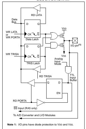
FIGURE 9-2: RA4/T0CKI PIN BLOCK DIAGRAM
