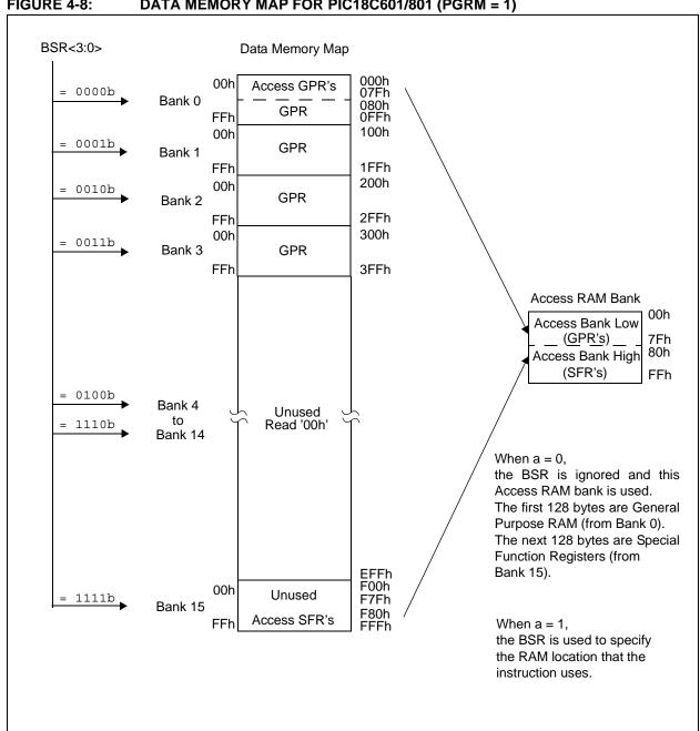
**FIGURE 4-8:** DATA MEMORY MAP FOR PIC18C601/801 (PGRM = 1)
