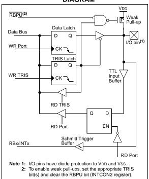
FIGURE 9-5: RB3 PIN BLOCK DIAGRAM
