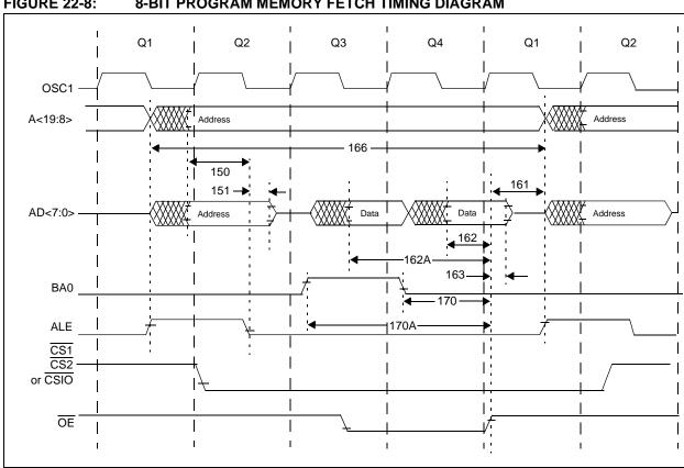
**FIGURE 22-8:** 8-BIT PROGRAM MEMORY FETCH TIMING DIAGRAM
