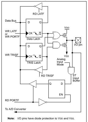
FIGURE 9-12: RF5:RF3 PINS BLOCK DIAGRAM
